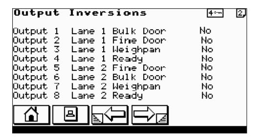
This screen allows the sense of each individual digital output to be inverted. Use the ENTER key to toggle between YES/NO.
