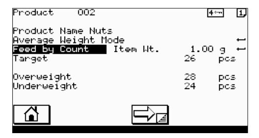
When the Count Option is Enabled (See Section **0 4.7.1 MACHINE SINGLE** / TWIN) then the **Feed by Count** option may be selected within the product setup. The entries below apply to **Feed by Count**.
