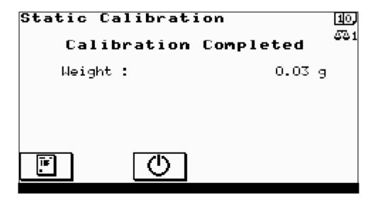
6. Check successful calibration by displayed weight agreeing with actual weight on weigher.
