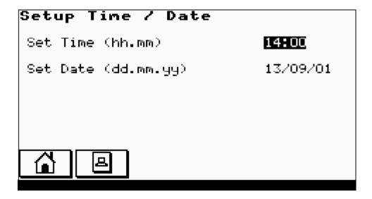
Setup current time and date. The system clock is battery backed and will maintain the correct time even when the machine is switched off.
