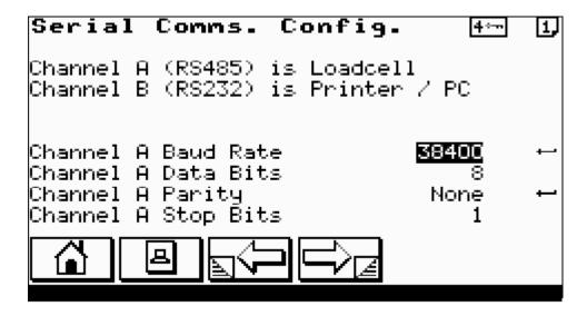
For each of the serial communications channels shown, setup the following parameters.
