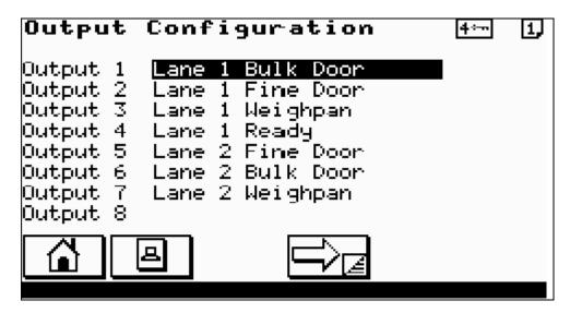
This screen allows each digital logical output to be assigned to a physical output. Use the ENTER key to select the logical output and the UP/DOWN ARROW keys to select the physical output.
