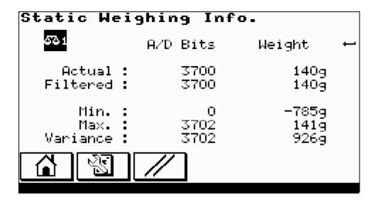
Shows current state of the loadcell a/d output and its conversion into weight.
