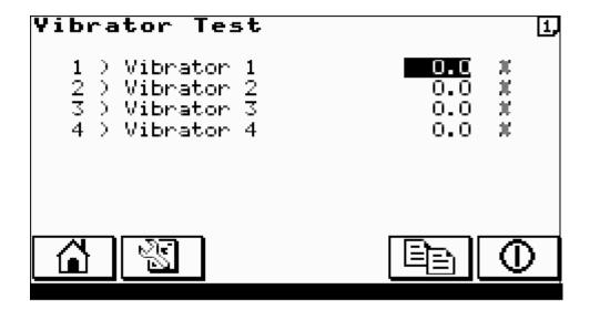
Enter test vibrator amplitudes.
