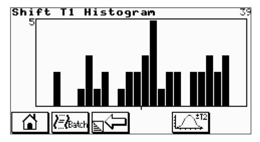
Shows weight histogram for batch or shift. Use batch/shift button to move between the two statistic sets. Use T1/T2 button to select histogram spread displayed.
