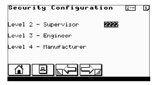
This screen can only be selected by the current level 4 password holder. Enter or reassign the password level codes.
