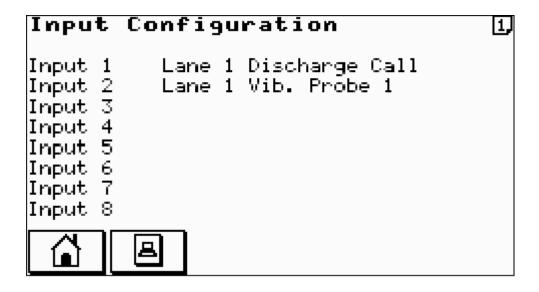
This screen allows each digital logical input to be assigned to a physical input. Use the ENTER key to select the logical input and the UP/DOWN ARROW keys to select the physical input.
